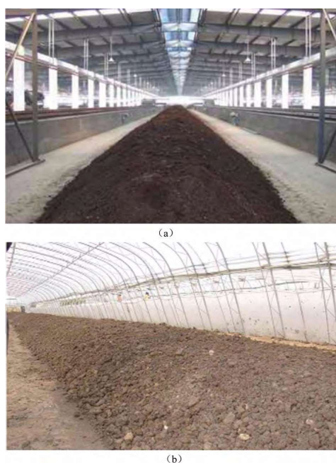
Figure 4. Strip stack composting.
