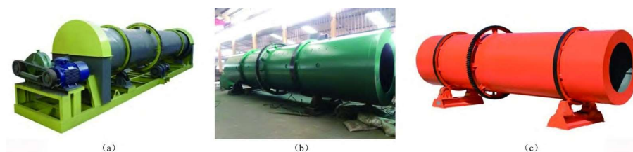
Figure 14. Rotary roller granulator.
