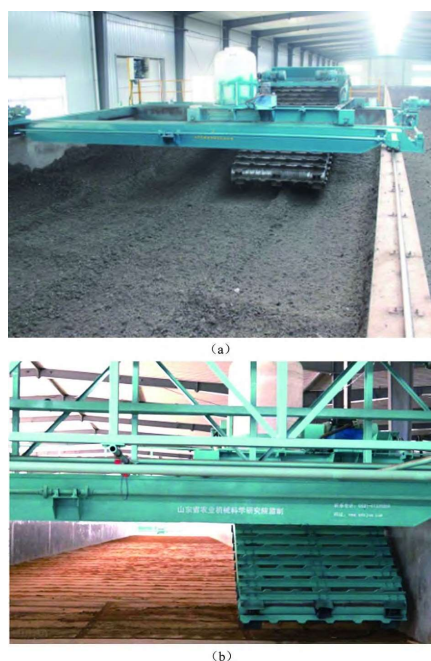
Figure 9. Trough-type composting wide chain plate turning and throwing machine.
